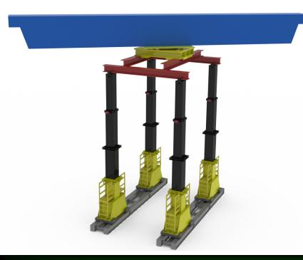
The Rotation Station makes it possible for the object to be rotated to be placed on top of the unit for 360 degree continuous rotation.
