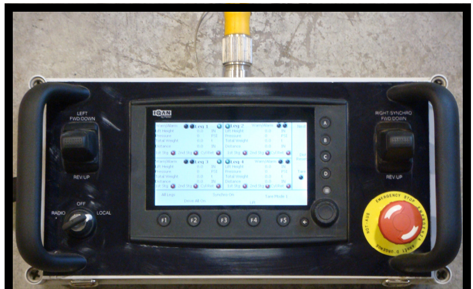
CONTROL MODULE FOR POWER TOWER
